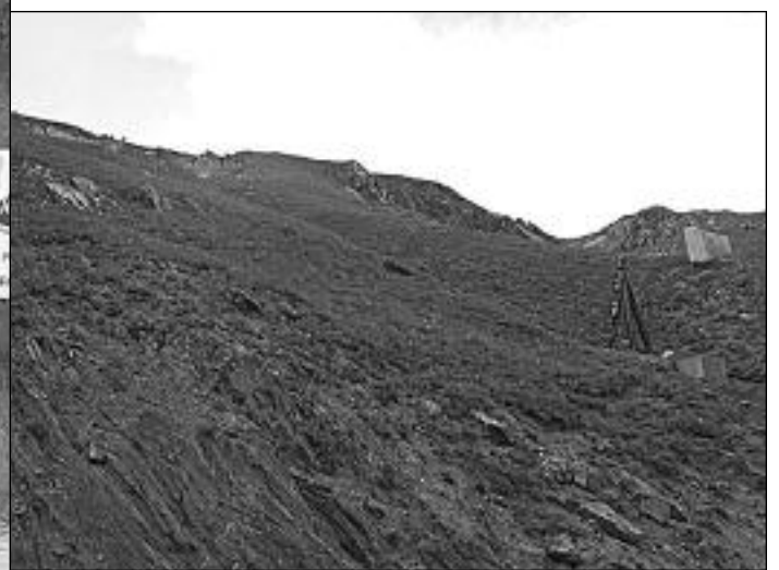
The CEMAGREF study site at Lauteret. Slides are triggered by Gazex or Avalex. Instrumentation can be attached to masts which run down the slope for several hundred meters. The instrument shelter is right on the roadway, chiseled into the bank. Photo by Mark Muller
