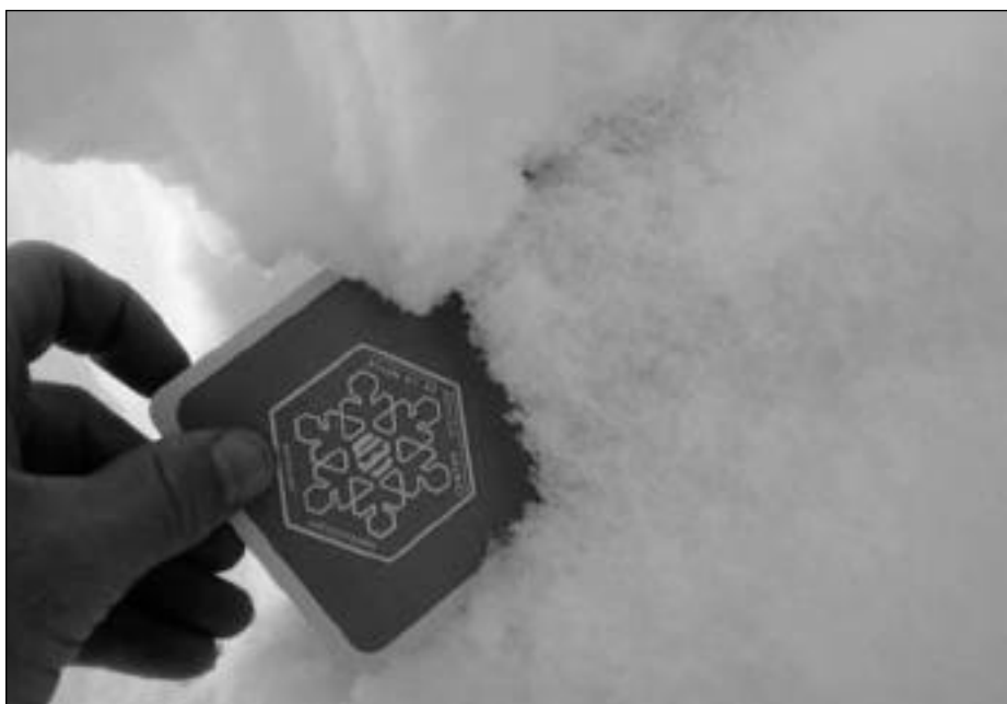
The tricks of the trade applied: this thick layer of faceted snow provided a very active layer for both natural and human triggered avalanches throughout the 2002-03 winter. Bruce Tremper photo (U.S. Forest Service Utah Avalanche Center).
