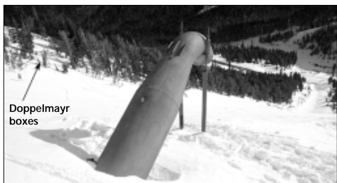
A Gazex tube sits poised over the Twin Slides starting zone. Doppelmayr Avalanche Guard boxes are indicated by the arrow. Two infrasonic sensors tuck into the trees at the middle left and lower left of the avalanche path. photo by Evan Howe
