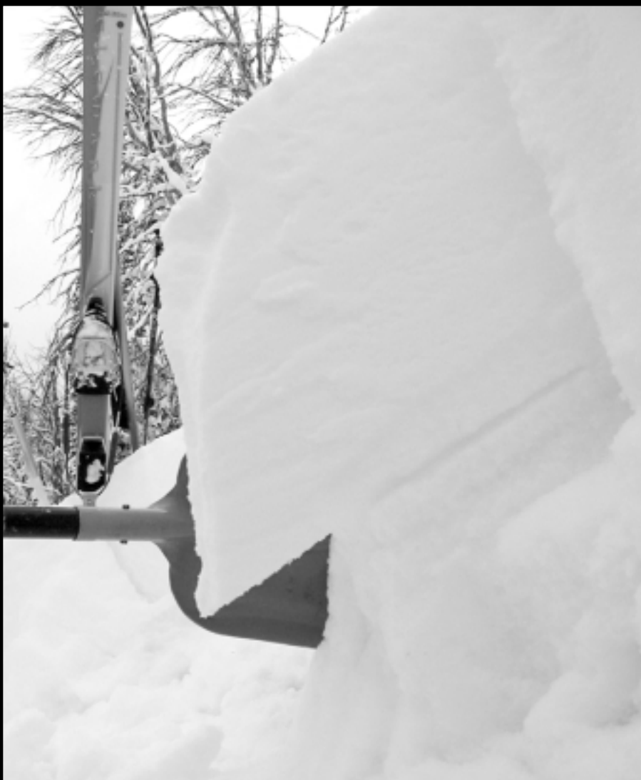
Examining the quality of shears can help to reduce uncertainty associated with variable stability test scores. Here a Q1 shear shows clean displacement of the slab. photo by Doug Chabot
