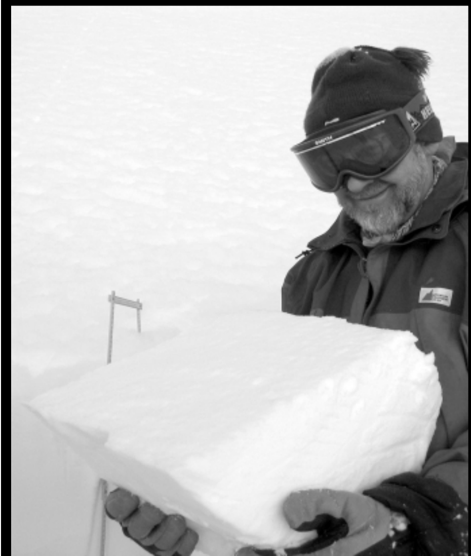
Dave McClung examines the shear quality and fracture character of a stability test. Cariboo, Canada. photo by Karl Birkeland/NAC
