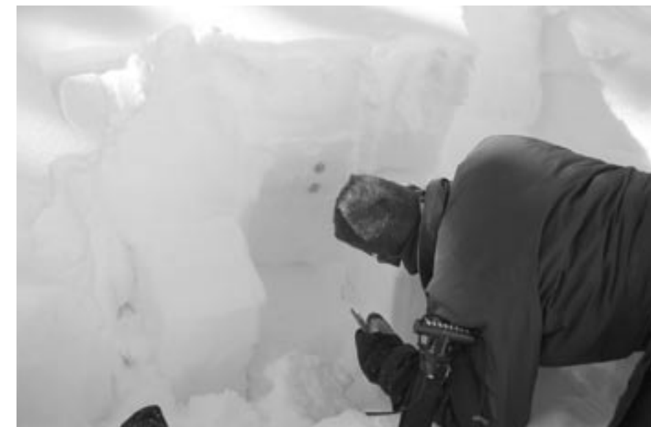
Craig examines a persistent weak surface-hoar layer in a pit off the Mirror Lake Highway.
