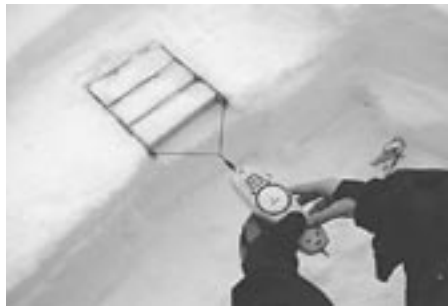
Shear Frame Test
