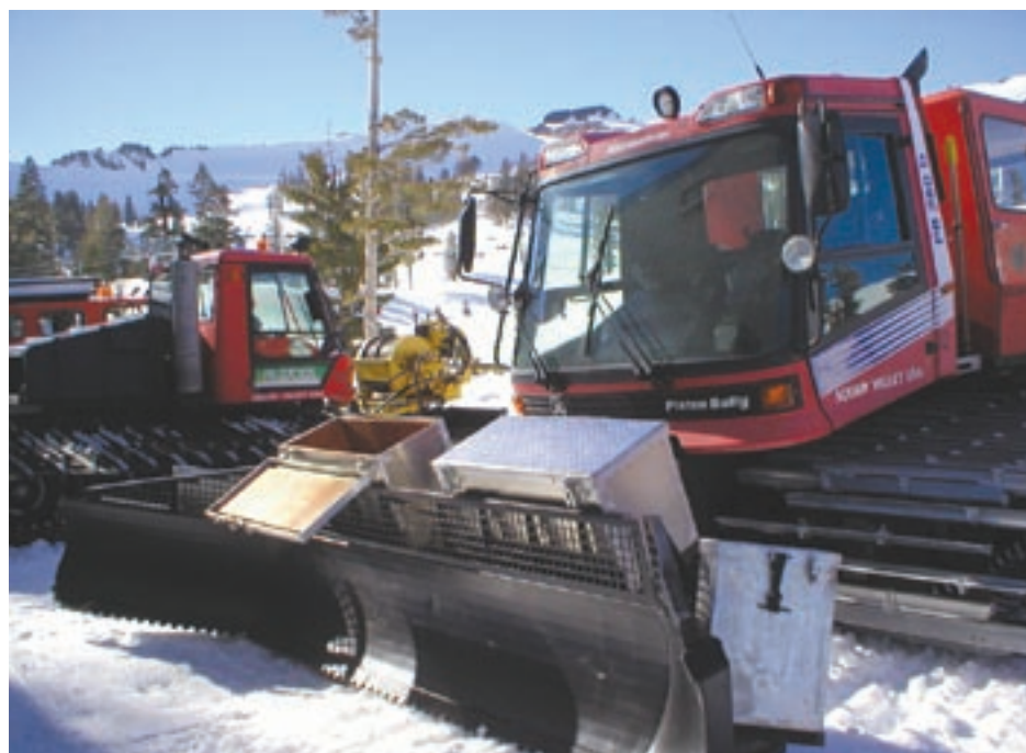
Unarmed charges are kept in their boxes and transported by cat to be armed on the hill. Trooper carriers now feature non-sparking interiors and wood-lined type-2 magazines on the front blades.
