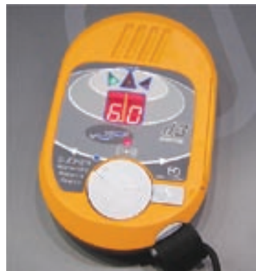
The Ortovox d3 transceiver has three antennas, is completely digital, and adds an LED to indicate if there are multiple signals.
