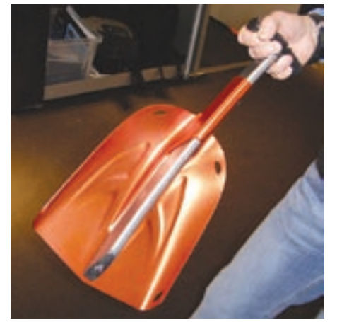
Black Diamond Deploy has a curved handle which slides over the blade for storage and prevents the shovel from spinning around while digging.
