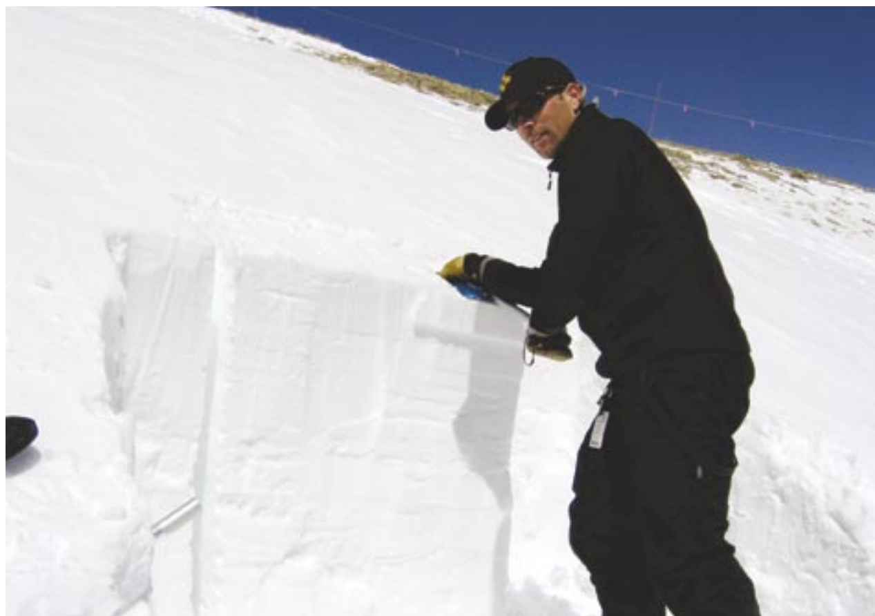
Fracture initiated but didn't propagate beyond the boundary of the loading area (shovel).
