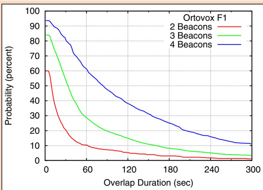
Figure 8. Probability of obtaining an overlap of specified duration for combinations of two, three, and four Ortovox F1 beacons.
