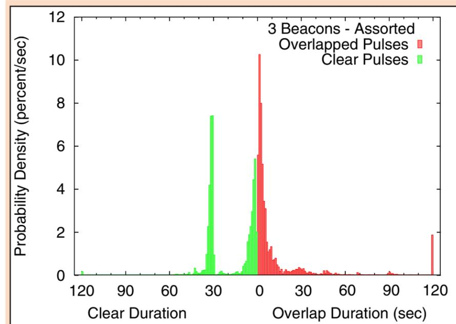
Figure 5. Histogram of overlap and clear durations for all possible combinations of three beacons taken from the study of Eck, et al.
