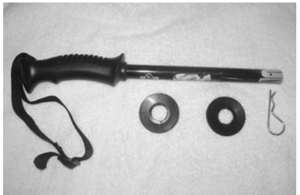
An old aluminum ski pole with a good strap, two fender washers, and a hairpin clip is all the materials you need to craft up a handy det cord roller. Cost: less than $2.
