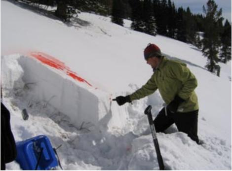
Figure 4. Author in Beehive Basin, MT pointing to dyed water coming out the pit wall after running along a capillary barrier located ~7cm from the surface. Photo by Karl Birkeland, National Avalanche Center
