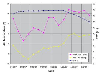
Figure 2. Graph detailing air temperature and SWE from 14 days before to wet-slab event. Data are from the NRCS Lone Mountain SNOTEL site, which is location approximately 400' below the crown of the slide.
