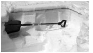
Figure 5: Meltwater accumulation along a surficial stratigraphic interface. Powdered dye was applied to the surface prior to the daily melt cycle.
