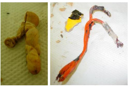
Left: The balloon that contains the sensitizing compound for the bulk of the cast shot was found about 30 feet from the blast crater. Notice the striations left from the rubber band. Right: The thawed out cap/fuse assembly clearly shows the end of the blasting caps where they are crimped to the fuses as well as at least an inch and a half of the cardboard tube detonator wells – showing that the detonators were properly installed.
