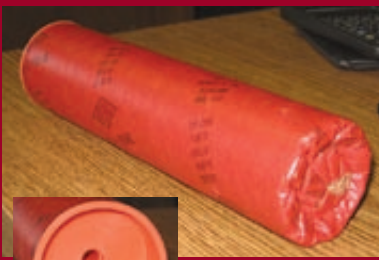
▲ Emulsion Hand Charges with cap wells
