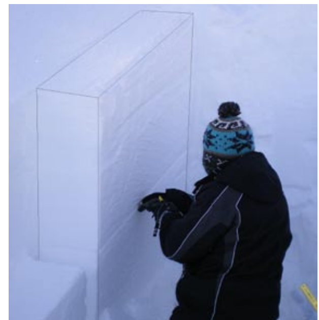
Fig 6: PST cutting in the uphill direction a long weak layer with the snow saw's none-serrated edge. Photo courtesy ASARC
