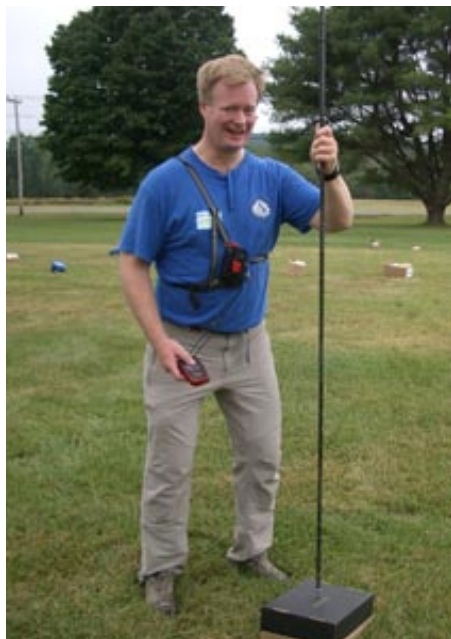
Mark Renson (Mad River Glen and Mount Washington ski patrols) uses his beacon and the new Pieps iProbe to find a "victim."
