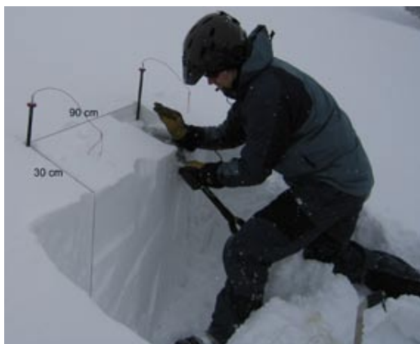
Fig 1: Jordy Hendriks demonstrates an ECT. The 90cm by 30 cm column oriented across the slope was cut with a cord and two probes. Photo by Karl Birkeland
