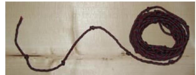
Fig 3: the tool of choice for most cases: a cord with knots every 10 – 20 cm.
