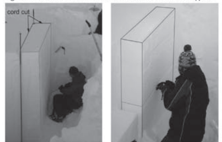
Fig. 2: Isolating a PST column (left) and saw-cutting upslope along the weak layer with the blunt edge (right).
