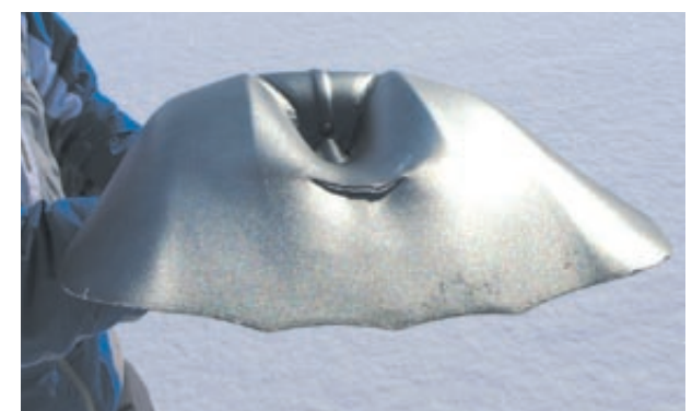
Despite its tough moniker, the Ortovox Grizzly cracked under the pressure of field testing. The serrated front blade edge, however, was given high marks for excellent cutting characteristics.
