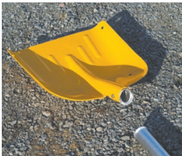
During testing, the BCA's shaft bent near the blade attachment until it finally snapped off completely.
