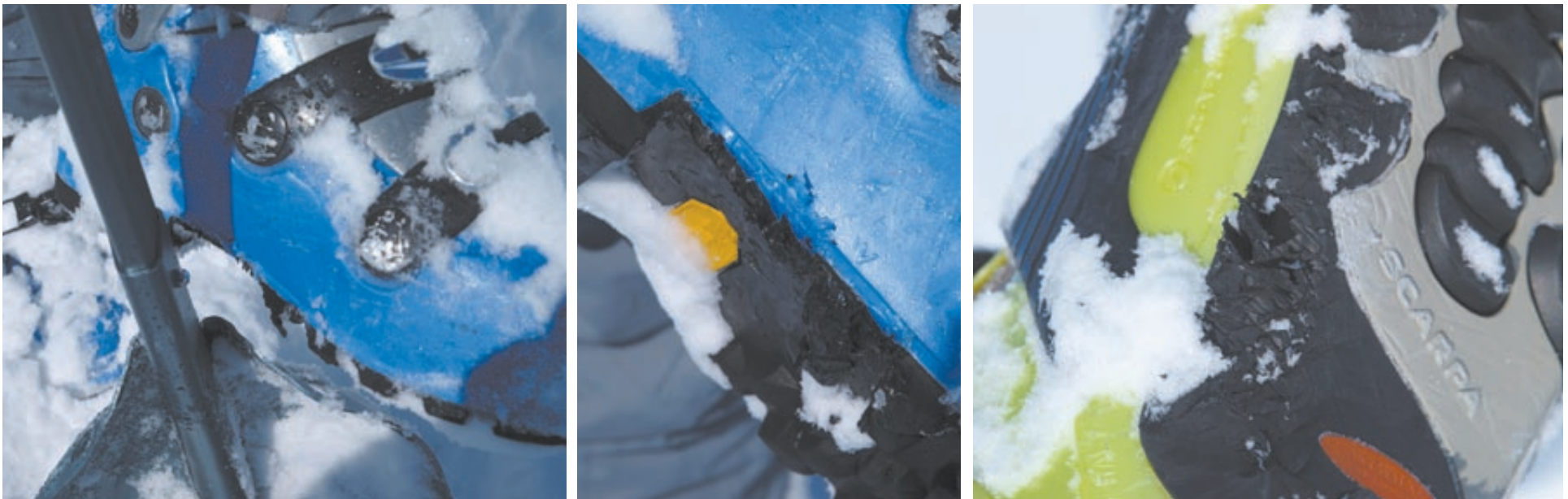
The shovel and the damage done: Several testers experienced severe damage to their ski boots, produced by the sharp edges and corners on top of Black Diamond's Transfer 7 shovel blade.
