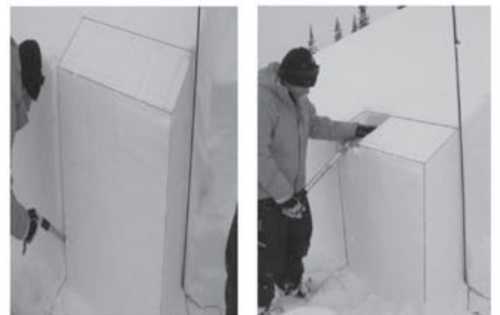
Fig. 2: Isolating an ECT column (left) and loading the column in the same manner as the compression test (right).
