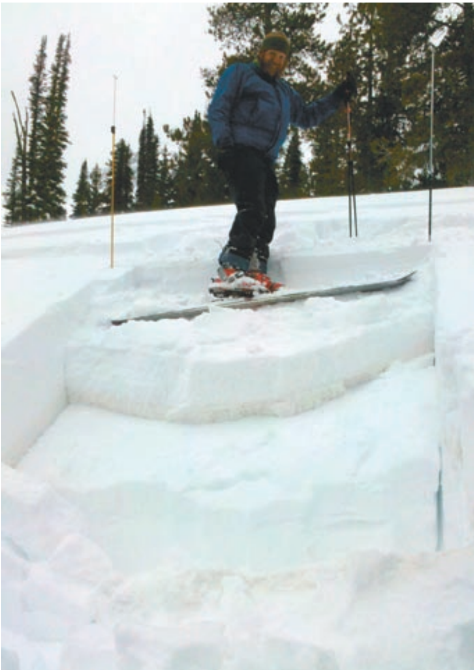
A dust layer above the MLK crust/ facet combo makes it easy to identify the culprit. A dense slab over the dust caused widespread failure on the MLK layer during the first week of March. Photo by Dave Bingaman
