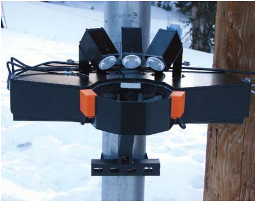
Installed at Alta Ski Area (far left), the three-pronged cameras of the MASC system capture images of snowflakes in free fall (right), allowing for detailed understanding of snow crystals and the layers they subsequently form.
