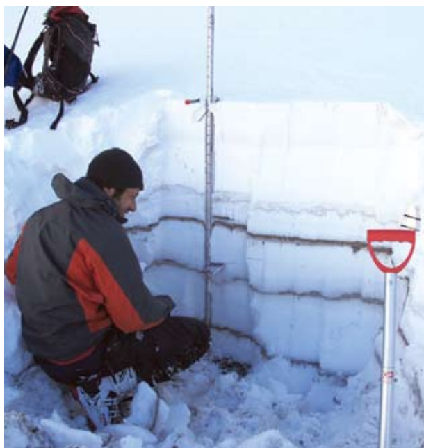
A snowpit converted into SnowPilot gives another set of evidence that although distinctive and abrasive, the ash layers were well-bonded to the rest of the pack.
