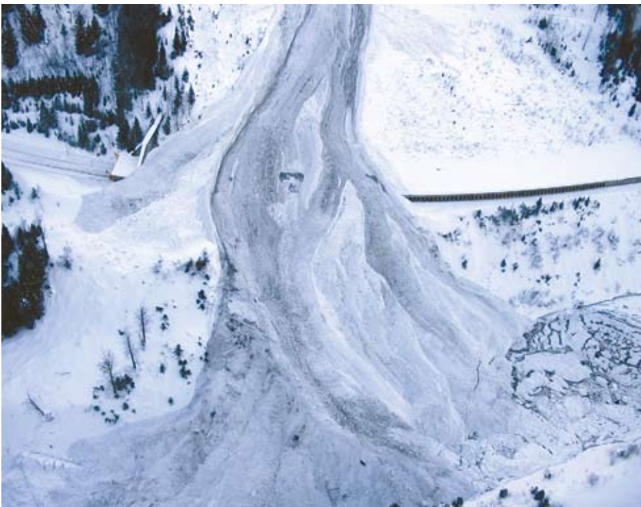
Lanark path, Rogers Pass: 8am, January 18, 2011. The avalanche was size D4.5 and damaged 10 acres of forest. It failed on facets/crust at ground. The air temperature dropped from -3°C to -17°C overnight prior to the event. The avalanche cycle was considered to be over. This one failed near the time that sun first hit the slope.
