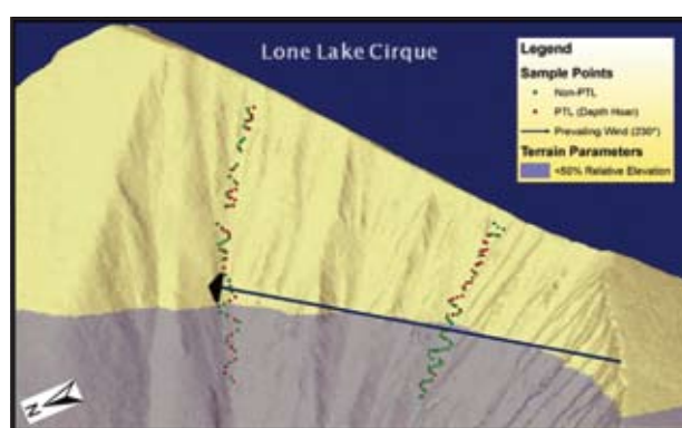
Figure 5: Distribution of depth hoar potential trigger locations (PTLs) in Lone Lake Cirque, illustrating how the influence of slope-scale parameters, such as relative elevation, depend on the broader-scale influences.
