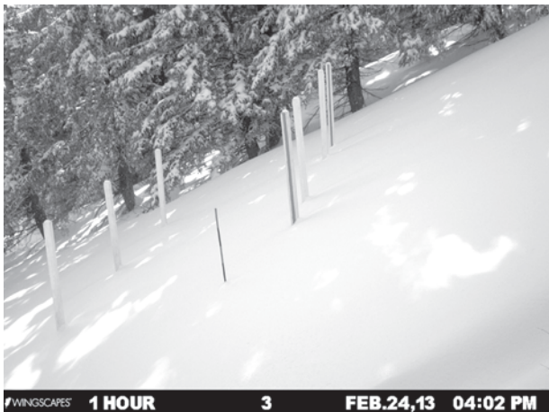
Sample image of the two depth markers deployed at the Bogus Basin snow study site. The white posts are cemented and mark the boundaries of lysimeters used to measure snowmelt.
