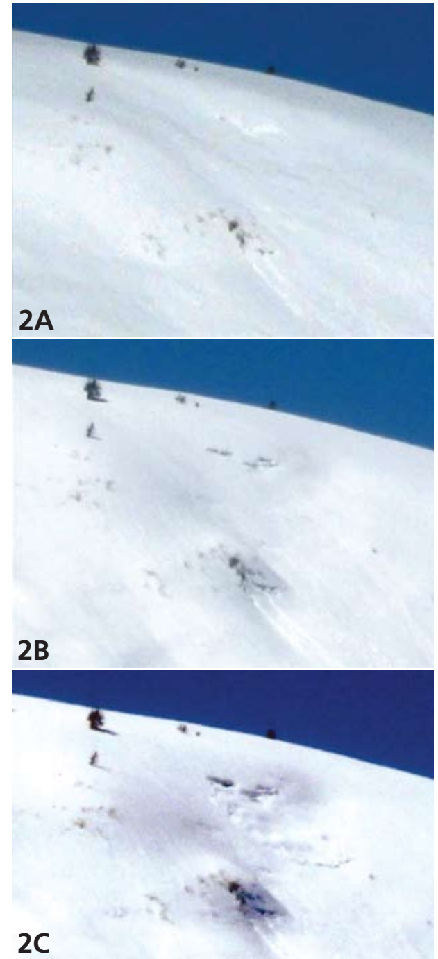
Figure 2: A sequence of three images showing the glide crack development before the avalanche on 28 April 2011. The last image is the last time-lapse image (>60) seconds before the avalanche released. The development of the staunchwall before the avalanche release is clearly evident in this picture.
