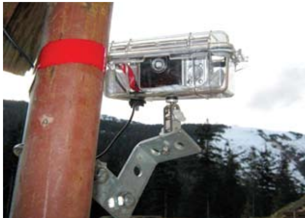
Figure 1: One of the Canon PowerShot A470 in the Kakuhan Mountain Range, Southeast Alaska. This camera was running on a hacked firmware and a time-lapse script.
