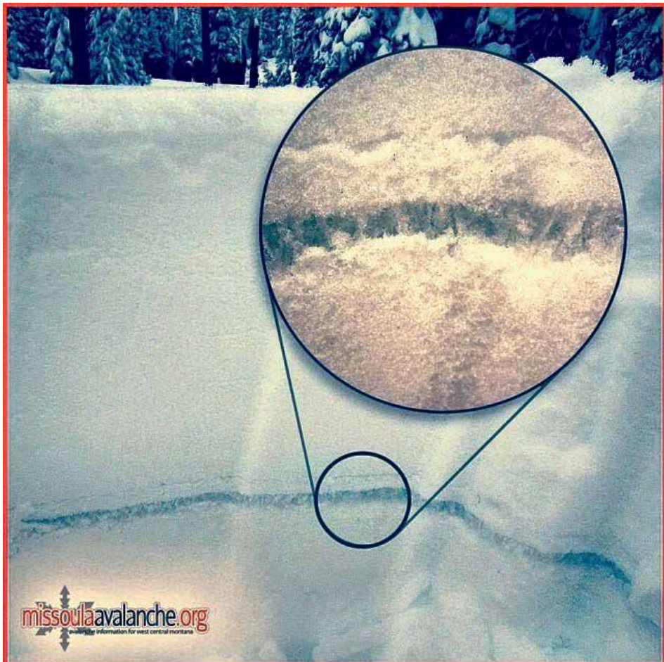
Surface hoar was created during the extended high pressure in January. The photo shows the layer buried in the Feb. 2 snowpack with a close-up and an avalanche class in the background. The pit is in our study plot near the Snowbowl Ski Area (Rattlesnake Mts. near Missoula). Photo by Dudley Improta
