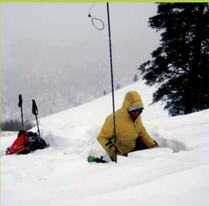
Dudley working up the crown profile on SE corner of crown. Photo by David Williams
