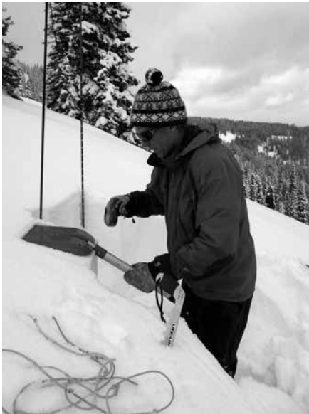
Figure 1: Collecting CT and ECT data (Dataset 1) on varying slope angles at our Lionhead study slope in Montana. Here our tests fractured on a buried layer of surface hoar with crystal sizes ranging from 6 to 15 mm. The grid size on the snow card is 2 mm.
