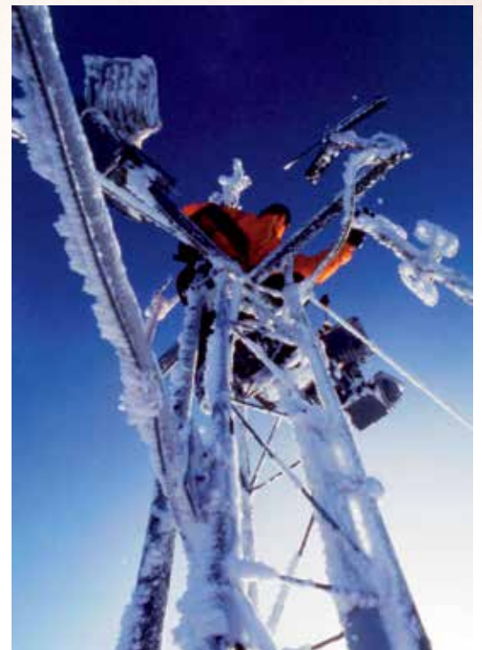
Back in the days before rime-free anemometers. De-riming the cups on top of Hidden Peak at Snowbird. Photo John Collins
