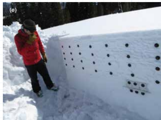
FIGURE 3: 30 cm long plastic supports inserted into the weak layer to arrest fracture in a PST. Reprinted from Birkeland et al. (2014b).
