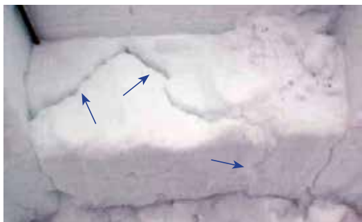
FIGURE 3: Post blast ECTN with top of column removed. These cracks were evident before I isolated the ECT column.
