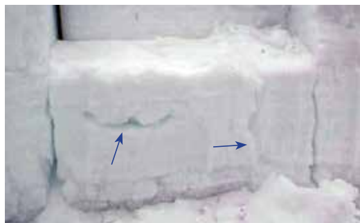
FIGURE 3: Post blast ECTN with top of column removed. These cracks were evident before I isolated the ECT column.
