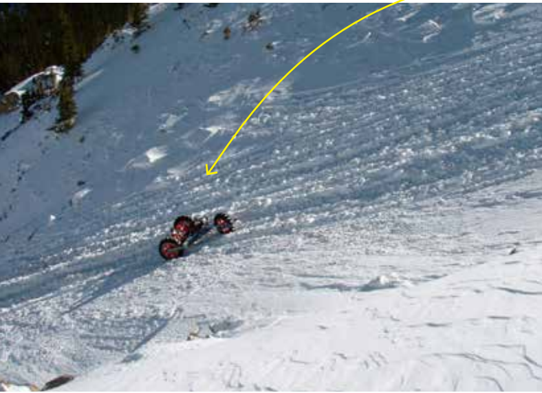
Winch roller compacting avalanche terrain Winter Park Resort, Winter Park, CO. Photo Mike Schneider
