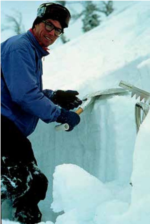
Karl conducting a compression test (with a bit of a sloppy pit wall!) around 1990. Photo Lonnie Ball
