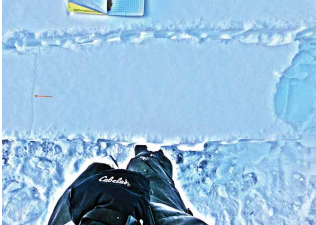
The rarely seen ECT slab fracture ~ 70 cm from the left edge of the shovel on a 3 m ECT. Contrast has been enhanced in this image.
