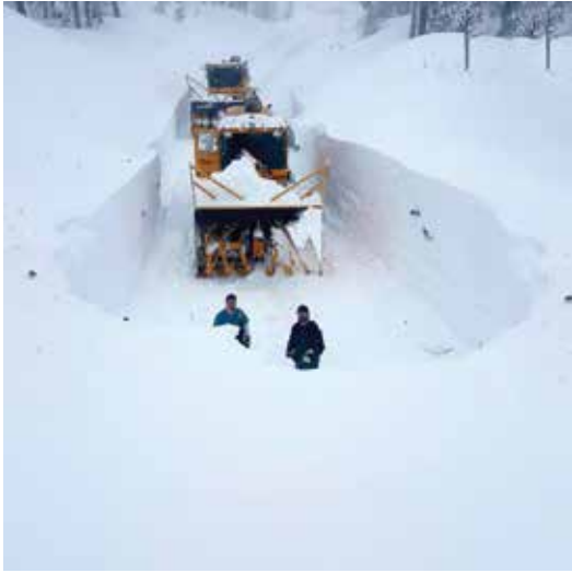
Mt. Rose: Blower operators foiled on the Slide Access Road as old growth trees and a lot of snow broke numerous sheer pins. Photo Dave Hahl
