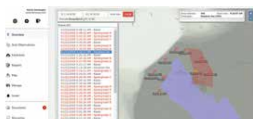
Figure 3: Integration of remote avalanche control systems (here "Sprengmast") and geophone and radar (blue areas) detection systems in one user friendly web-platform.
