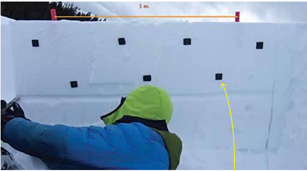
Figure 3: Pit setup with a tilted camera in the slope direction to capture the slab sliding motion in the x-axis. The red markers on the top of the PST-like block are 1 m apart for size calibration. The black rectangles are used by the tracking software as a reference point to measure motion for every video frame.
