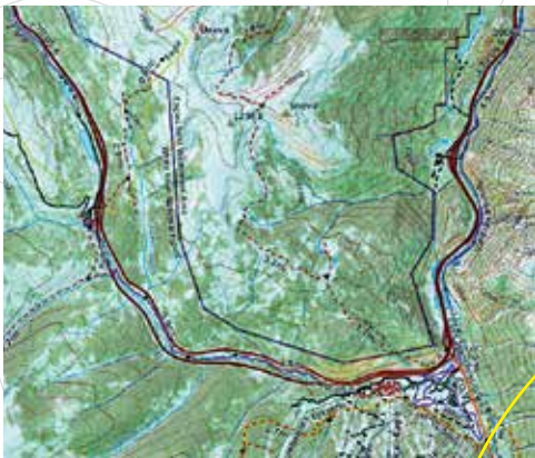
False Color Green Sentinel imagery stacked on top of MapBuilder Topo provides current snow coverage information with topographic data to reference.
