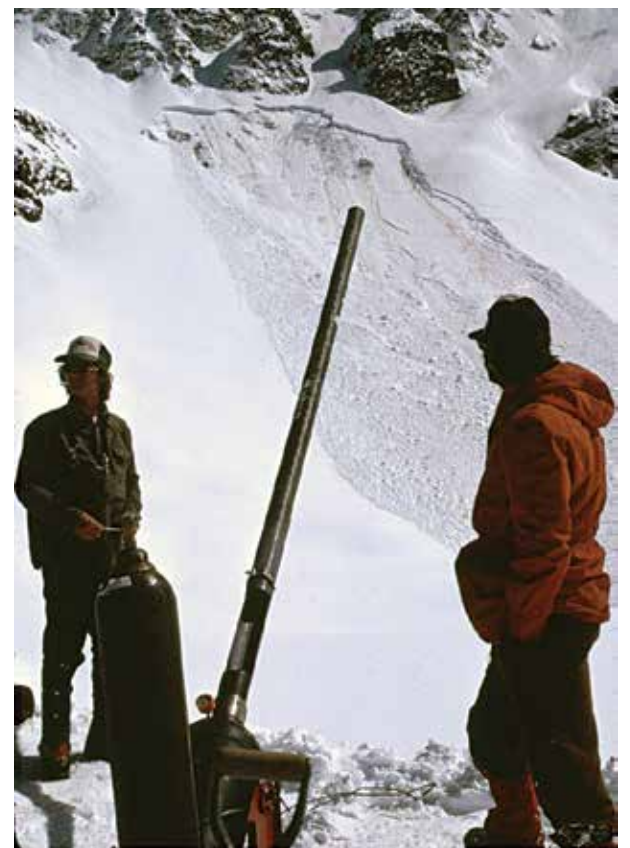
Next! Using the avalauncher to protect the Silverton speed skiing venue in 1983. Photo Don Bachman
