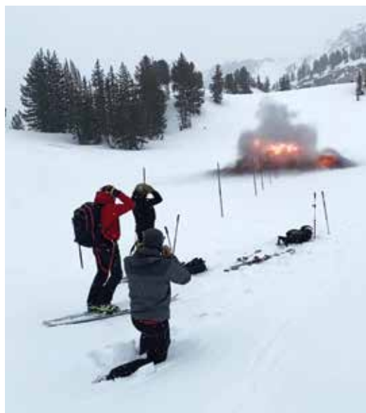
Counter-clockwise from top: Controlled test using pressure sensors. Sensors are attached to bamboo at known distances to measure the decay of the pressure wave as it spreads out from the point of detonation.
